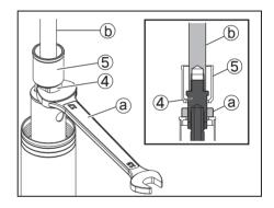
6. Pull up the tool ⓑ to remove the wrench ⓐ, and remove the tool ⓑ and slider ⑤.
