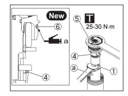
6. Clamp the part C of outer tube ⑦, and attach the fork bolt COMP ⑤ using a tool with the specified torque.
