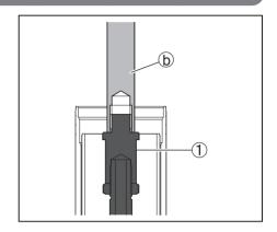
2. Attach the spring collar COMP 2 and the slider 3.
