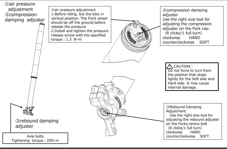
Manual for A-Kit RC For details of removing and mounting, please refer to the 18YM CRF450R Owner'S/ Service Manual of the motorcycle manufacturer.
