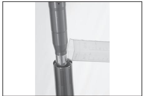
15. Apply grease on a new O-ring ①, and attach to the groove part ③ of the damper COMP ②.
