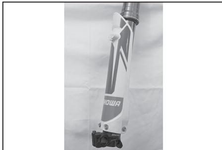
6. Attach the front wheel ①, brake caliper ②, and brake hose ③.
