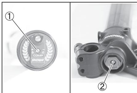
4. Clamp the outer tube ① on the [C] part, and remove the cushion S/COMP ② using the special tool.
