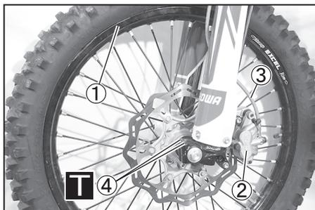
7. Tighten the screw ④ of the axle holder with the specified torque.
