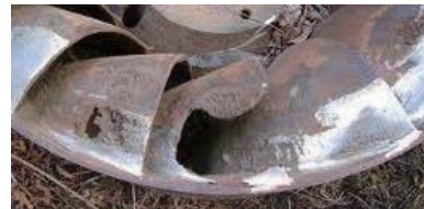
Marine propeller eroded by cavitation
