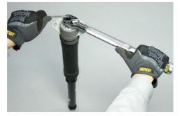
Then, reassemble parts in the reverse order as they were attached. Then, reassemble parts in the reverse order as they were attached. Make sure that the upper mount and the lower bushing are facing in the right direction, then fasten the upper nut with a prescribed torque
