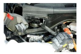
Reinstall the strut assembly into the vehicle in the reverse process. Torque control is always required when tightening bolt and nut
