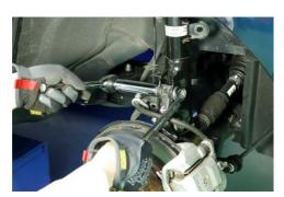
Tighten the nuts and bolts that are holding the strut lower bracket, just for temporary
