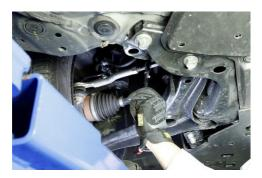
Adjust the toe-in with a tie rod on the front left wheel. First, loosen the locknut and turn the rack end. After adjusting, fasten the locknut with a right torque.
