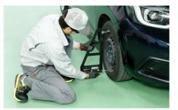
Make sure that the camber angle is correct with camber gauge
