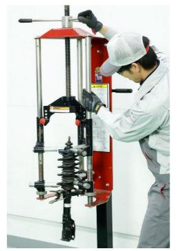
After removing the center nut, pull the strut out from underneath and check the spring seat mount, dust boot, and bump rubber for cracks or fatigue
