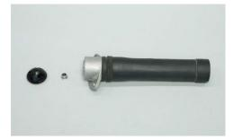
Check the structure for the correct direction of the upper mount, washer, collar, dust cover, and bump rubber, and then remove each part from the shock absorber. Make sure all parts have no damages or worn
