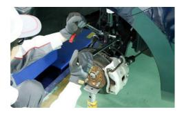
After removing the brake hose and others, loosen the nuts and bolts that are holding the strut lower bracket
