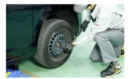
Install tires and tighten the wheel nuts with correct torque while lowering the hoist until tires are fully grounded
