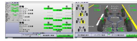
After adjusting the tie-rod, set computerized wheel alignment equipment again and measure the toe-in one more time. Make sure that the toe-in amount is within the correct range
