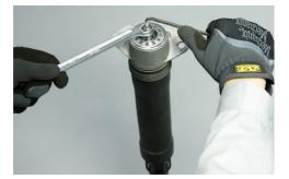
Loosen the shock absorber upper nut a while holding the flat face or hexagon hole on the top of rod with suitable tools
