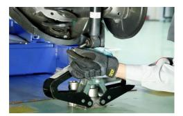
Loosen the lower nut and bolt on the shock absorber
