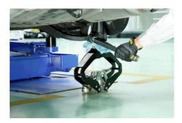
After hand tighten the bolt and nut at bottom side of shock absorber, applying 1G force by lifting jack up, tightening them with correct torque
