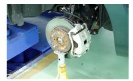
Once the strut knuckle bolts are removed, ensure that the steering knuckle and axle carrier are supported by the jack
