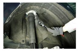
Remove the nuts /bolts from the upper mount
