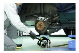
Insert the jack underneath rear axle carrier or lower arm
