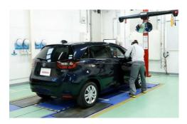
Move the vehicle back and forth to penetrate the replaced spring and the strut
