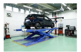
Now let's check the wheel alignment. Here is a typical computerized wheel alignment equipment to check the toe-in of each wheel
