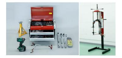
STD Tool Box Rigid Rack Steering Holder Torque Wrench Camber Gage Spring Compressor Impact Wrench
