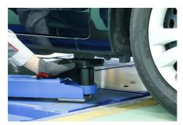
Raise the hoist a little to check that it is supporting the designated lifting points of vehicle correctly
