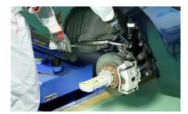
With adjusting to original camber angle, fasten the nuts and bolts that are holding the strut lower bracket with correct torque
