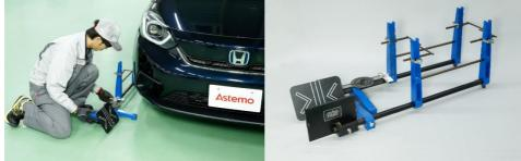
Even if computerized wheel alignment equipment is not available, toe-in/out can be checked with a toe-in gauge or sideslip tester
