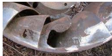
Marine propeller eroded by cavitation
