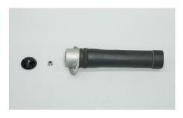
Check the structure for the correct direction of the upper mount, washer, collar, dust cover, and bump rubber, and then remove each part from the shock absorber. Make sure all parts have no damages or worn
