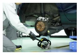
Insert the jack underneath rear axle carrier or lower arm
