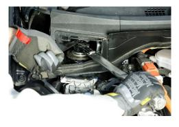
Reinstall the strut assembly into the vehicle in the reverse process. Torque control is always required when tightening bolt and nut
