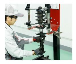
Mark the location of how the mount was seated before compressing the spring. Now you can compress the coil spring until there is a room between coil spring and mounting.
