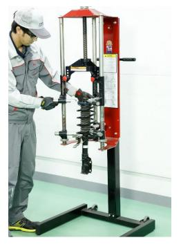
After removing the center bearing dust cap of the upper strut mount, set the strut assembly between the top and bottom of the coil spring to the spring compressor equipment
