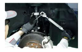
Depending on the vehicle, it might be required special tools to apply correct tightening torque
