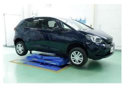
Then lift the car up until the wheel leaves the ground
