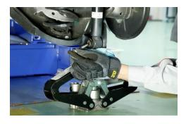
Loosen the lower nut and bolt on the shock absorber
