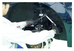
Remove all attached parts, such as the brake hose, sensors, and sway-bar, from the strut
