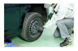
Install tires and tighten the wheel nuts with correct torque while lowering the hoist until tires are fully grounded
