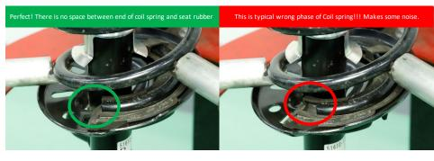
Place new strut on holder of spring compressor equipment with correct phase of coil spring
