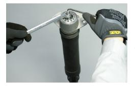
Loosen the shock absorber upper nut a while holding the flat face or hexagon hole on the top of rod with suitable tools
