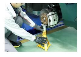
Insert the jack underneath to prevent the axle carrier from falling over. This will avoid any trouble with the driveshaft, wiring harnesses, or brake system
