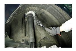
Remove the nuts /bolts from the upper mount
