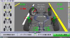
The wheel alignment equipment indicates that the left front wheel is toedin strongly in this case. The left front wheel toe needs to be adjusted
