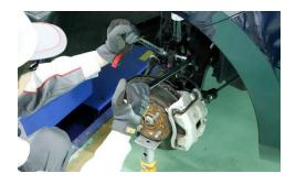
After removing the brake hose and others, loosen the nuts and bolts that are holding the strut lower bracket
