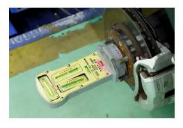
Check and record the camber angle before taking the suspension apart
