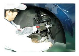
Pull out with the upper mount from the vehicle body, by shifting the strut assembly downward
