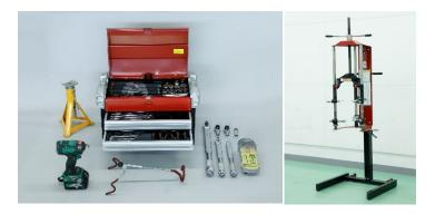
STD Tool Box Rigid Rack Steering Holder **Torque Wrench** Camber Gage **Spring Compressor** Impact Wrench
