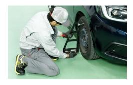
Make sure that the camber angle is correct with camber gauge
