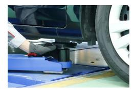
Raise the hoist a little to check that it is supporting the designated lifting points of vehicle correctly
