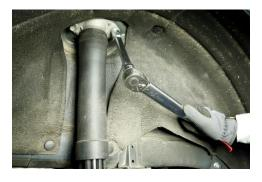
Reinstall the shock absorber assembly in the reverse order. Tighten upper nuts /bolts with correct torque
