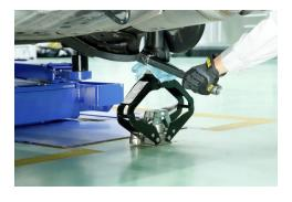
After hand tighten the bolt and nut at bottom side of shock absorber, applying 1G force by lifting jack up, tightening them with correct torque
