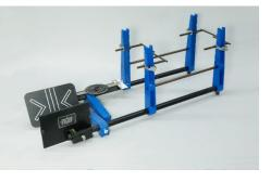
Even if computerized wheel alignment equipment is not available, toe-in/out can be checked with a toe-in gauge or sideslip tester
