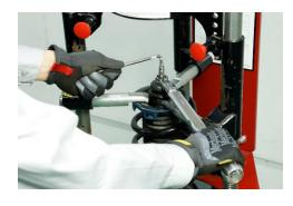
Fasten the center nut with the correct torque while holding the rod with appropriate tool
