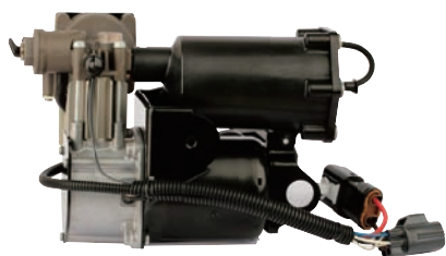
Air compressor for air suspension
