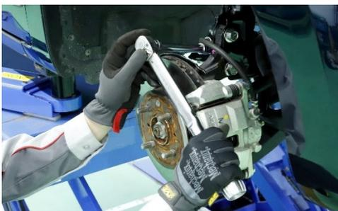
Put all attached parts, such as the brake hose, sensors, and sway-bar to the strut with correct tightening torque
