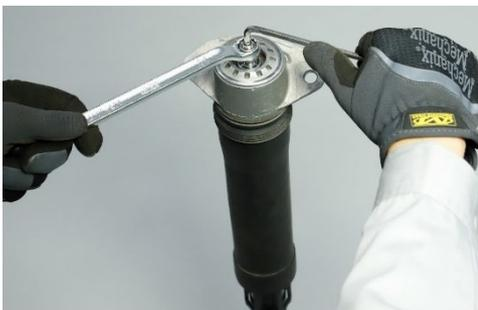
Loosen the shock absorber upper nut a while holding the flat face or hexagon hole on the top of rod with suitable tools
