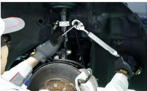
Depending on the vehicle, it might be required special tools to apply correct tightening torque
