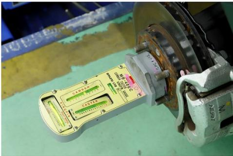
Check and record the camber angle before taking the suspension apart
