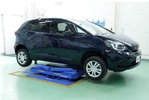
Then lift the car up until the wheel leaves the ground
