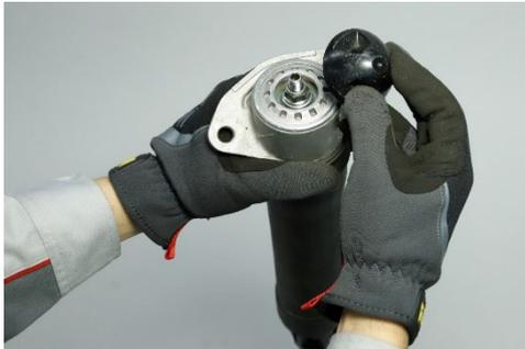
Make sure all parts were assembled to shock absorber, even plastic top cap
