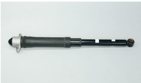
Remove the shock absorber assembly from the axle carrier, by lifting the assembly with your hands, and then remove it from the vehicle
