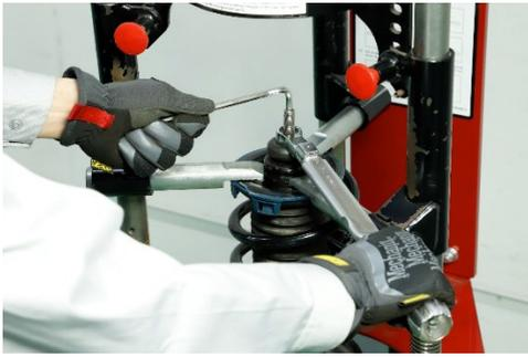
Fasten the center nut with the correct torque while holding the rod with appropriate tool
