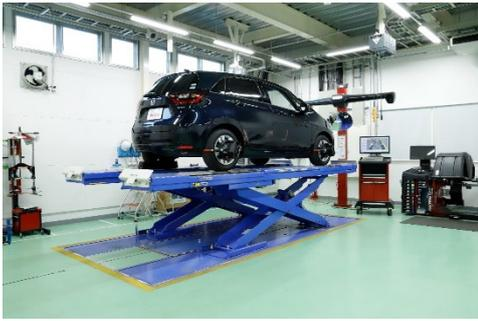
Now let's check the wheel alignment. Here is a typical computerized wheel alignment equipment to check the toe-in of each wheel
