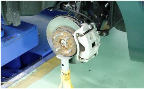
Once the strut knuckle bolts are removed, ensure that the steering knuckle and axle carrier are supported by the jack
