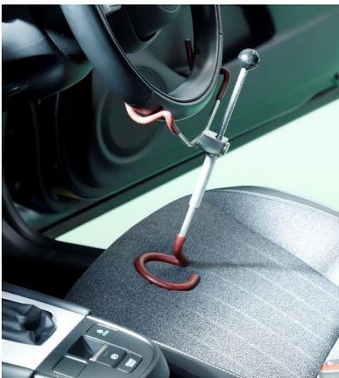
Using Steering wheel holder tool to prevent front tires from being steered
