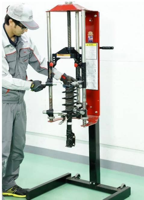
After removing the center bearing dust cap of the upper strut mount, set the strut assembly between the top and bottom of the coil spring to the spring compressor equipment
