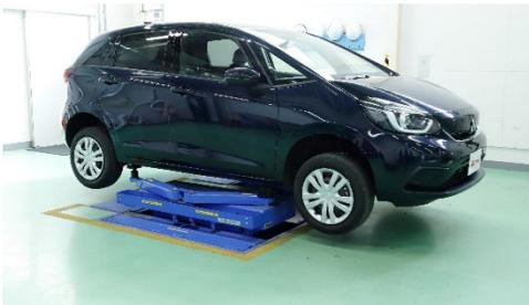
Then lift the car up until the wheel leaves the ground
