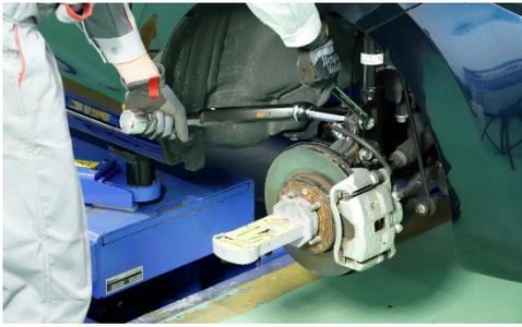
With adjusting to original camber angle, fasten the nuts and bolts that are holding the strut lower bracket with correct torque
