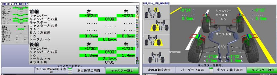
After adjusting the tie-rod, set computerized wheel alignment equipment again and measure the toe-in one more time. Make sure that the toe-in amount is within the correct range
