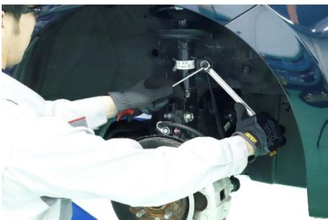
Remove all attached parts, such as the brake hose, sensors, and sway-bar, from the strut
