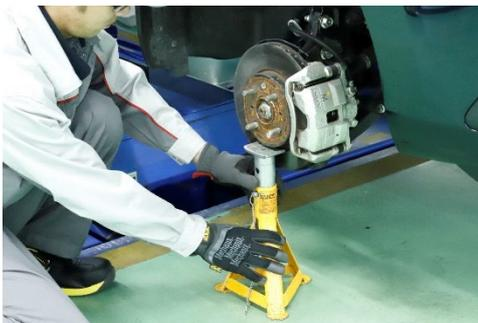
Insert the jack underneath to prevent the axle carrier from falling over. This will avoid any trouble with the driveshaft, wiring harnesses, or brake system
