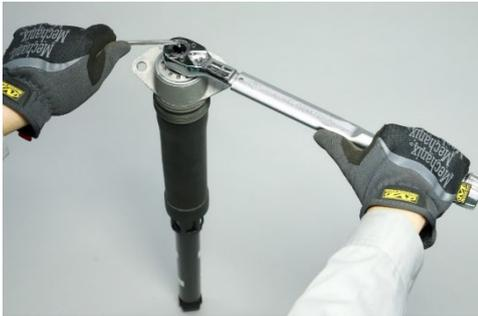
Then, reassemble parts in the reverse order as they were attached. Then, reassemble parts in the reverse order as they were attached. Make sure that the upper mount and the lower bushing are facing in the right direction, then fasten the upper nut with a prescribed torque
