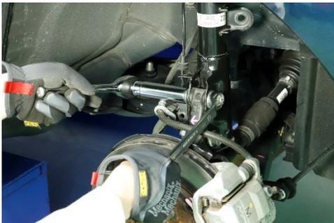
Tighten the nuts and bolts that are holding the strut lower bracket, just for temporary
