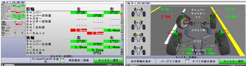
The wheel alignment equipment indicates that the left front wheel is toed-in strongly in this case. The left front wheel toe needs to be adjusted
