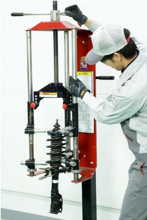
After removing the center nut, pull the strut out from underneath and check the spring seat mount, dust boot, and bump rubber for cracks or fatigue
