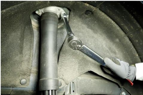
Reinstall the shock absorber assembly in the reverse order. Tighten upper nuts /bolts with correct torque
