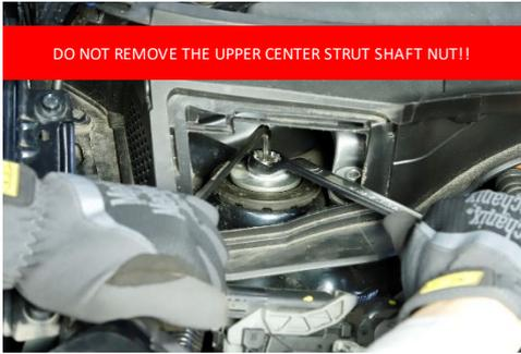
After opening hood loosen center shaft nut and remove the upper strut mounts nuts
