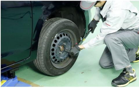
Install tires and tighten the wheel nuts with correct torque while lowering the hoist until tires are fully grounded
