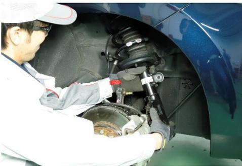
Pull out with the upper mount from the vehicle body, by shifting the strut assembly downward
